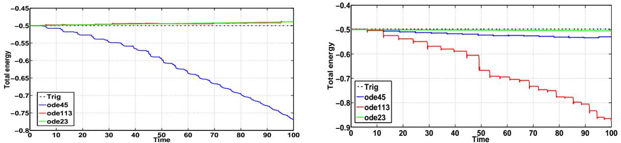
Figure 1: Total energy evolution for the two body problem using trigonometric interpolation with  $S = 5$  and  $h = 0.01$  compared with ode45, ode113 and ode23. Left: eccentricity  $\epsilon = 0.2$ . Right: eccentricity  $\epsilon = 0.8$ .
