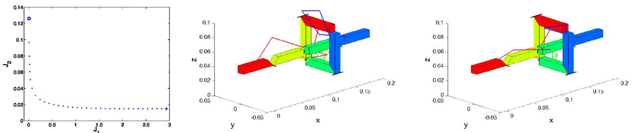
Figure 1: Left: Approximation of the computed Pareto front for the objectives  $J_1$  and  $J_2$ . Middle: Center of mass trajectories for the Pareto point ('o' in left). Right: Center of mass trajectory for the Pareto point ('+' in left).
