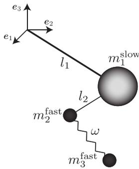
Figure 3: Example subject to constraints: triple spherical pendulum with slow and fast variables
