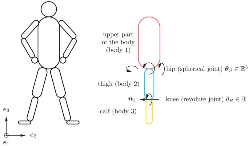
Figure 1: Model of the monopedal jumper.
