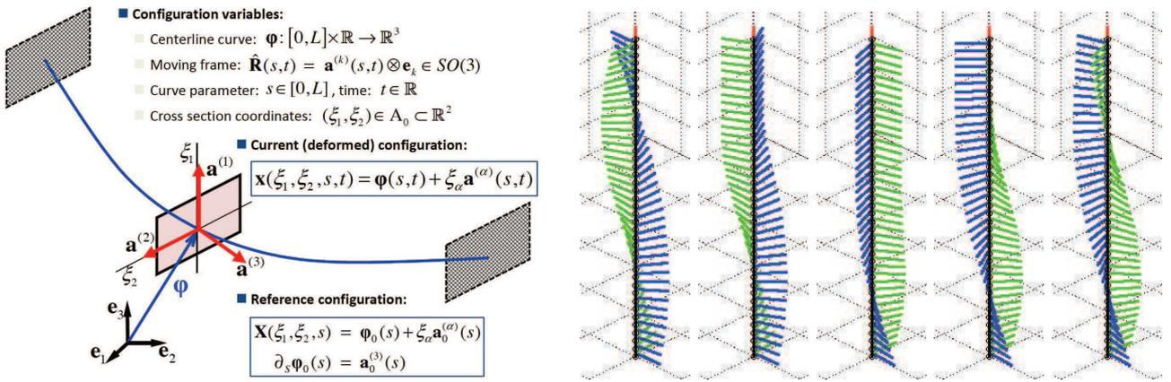
Figure 1: Left: Kinematic quantities for the (deformed) current and (undeformed) reference configurations of a Cosserat rod. Right: Snapshots of a purely torsional, slightly damped vibration of a cosserat rod, fully clamped at the lower end.
