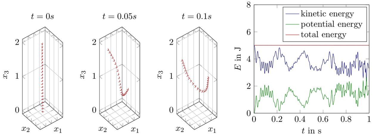
Figure 1: Simulation of a geometrically exact beam with momentum initial conditions using AVI. Left: Snapshots of the motion. Right: Corresponding energy plot with no numerical dissipation.
