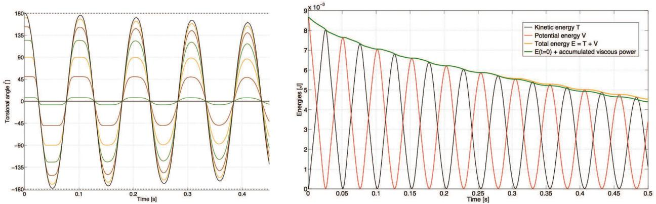
Figure 2: Left: Dynamic evolution of selected torsional angles for purely torsional vibrations. Right: Energies for damped torsional vibrations. The discrepancy between the total energy  $E(t) = T(t) + V(t)$  and  $E(t = 0) + \int_0^t P_v(\tau) d\tau$  with the viscous power  $P_v$  estimates the numerical damping of the underlying numerical time integration scheme.
