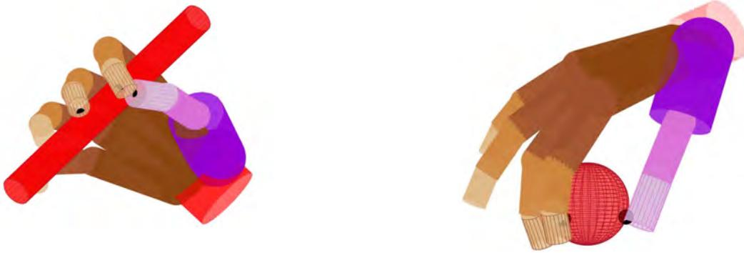
Figure 1: The final postures for grasping a cylinder (left) and a sphere (right) with 3 contact points. The hand is kinematically actuated through 5 synergies which control the 20 joint angles.
