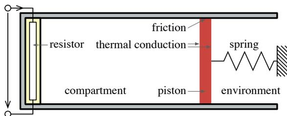
sketch of a piston-cylinder device
